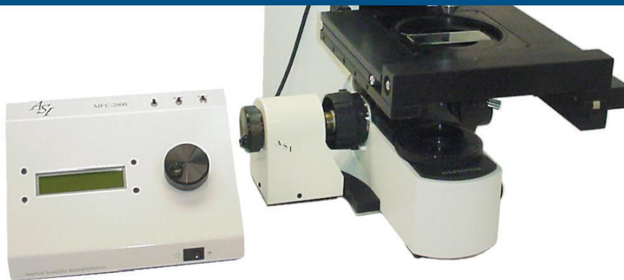
The MFC-2000 has been specifically designed to provide a high resolution and highly repeatable, means of controlling the focus/Z position of the microscope stage. Precise control of the microscope's focus is obtained through the use of a closed-loop DC servomotor employing high resolution encoders for positioning feedback. By using closed-loop control of the focus position, there is no chance that the focus point can be lost as can occur with open-loop stepper motors.
