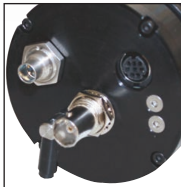
LDB100F Brightfield LED with flip-in 550 nanometer filter.
